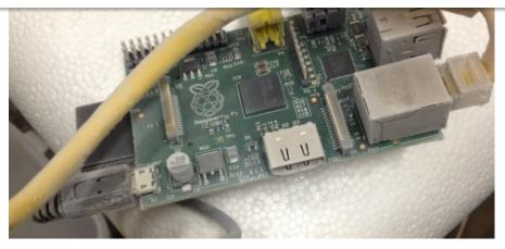
Once the tub was submerged, the temperature of the board initially dropped down to -78°C before it stopped responding. However, removing the board and replacing it after 30 seconds saw the temperature drop to -82°C and then -87°C before the Pi stopped working again. At its limit the Raspberry Pi continued to function right up to -110°C, and then started working again once it had warmed back up.
